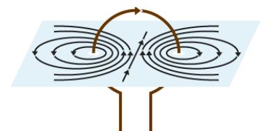
A **force** acts on a **current-carrying conductor** in a magnetic field.
