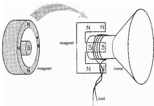
**Loud speakers** consist of a coil attached to a cone in a magnetic field. When **alternating current** flows through the coil, the cone is continuously pushed away and pulled back, making a **sound**. The **frequency** (and therefore pitch) of the sound can be altered by changing the frequency of the alternating current used.
